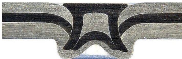
Figure 12: rivetage autopoinçonnant (source: Henrob innovative joining solutions)
