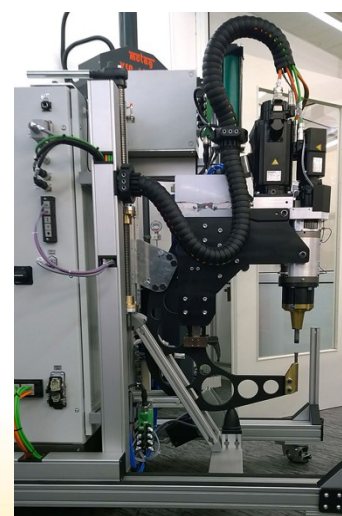
Figure 6: soudeuse friction spot
