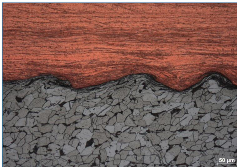
**Figure 23 :** Wavy weld interface of a copper-steel weld (detail of Figure 22)
