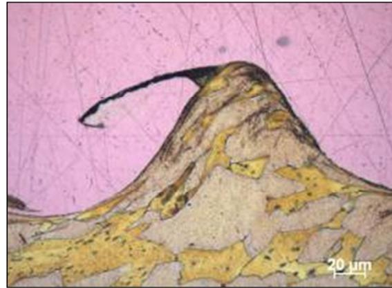
**Figure 18:** Cross section of a magnetic pulse weld of copper to brass - Detail of Figure 17 (Source: BWI-CEWAC project SOUDIMMA)
