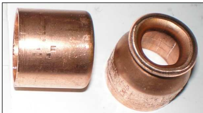
Figuur 10 : Resultaat van experiment C30_Cu_08 (voltage = 18,0 kV - 25,9 kJ).
