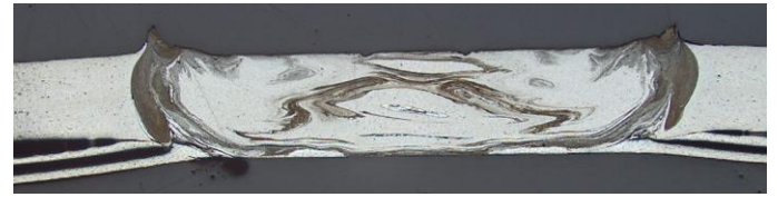
Figure 15: Typical cross-section, RFSSW on non-displaced MPC core.
