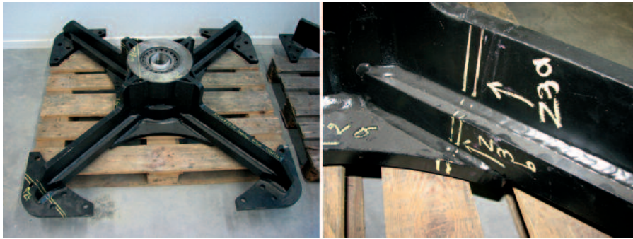
Fig. 7 • HF900 bearing house. Left: original design; Right: a detail of the critical point for fatigue crack initiation at the star-shaped reinforcement.
