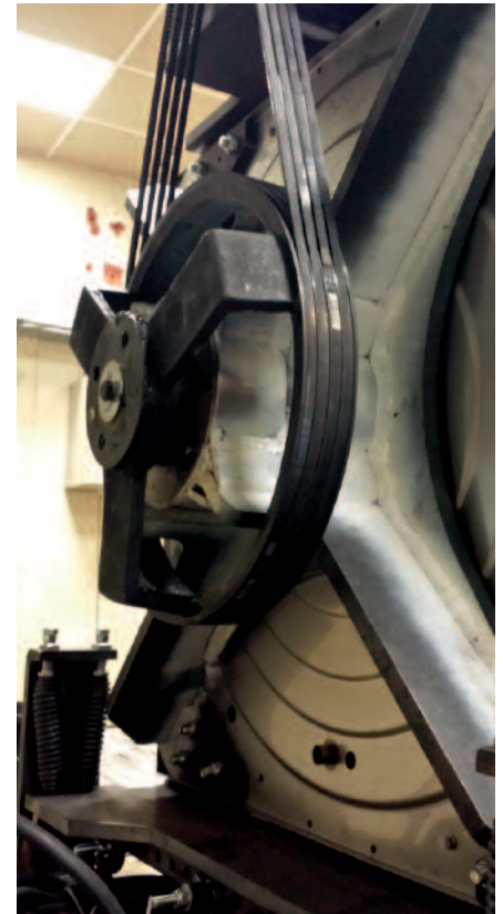
Fig. 6 • HF900 bearing house of an industrial washing machine ready for out-of-balance test.
