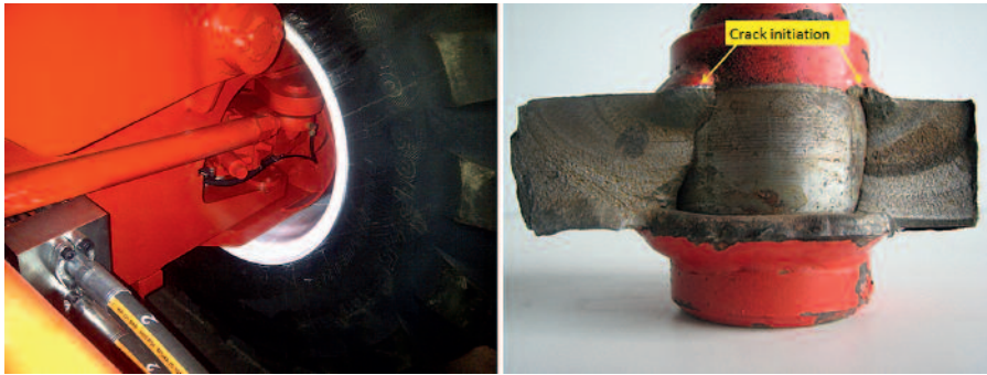
Fig. 4 • Steering lever. Left: location of the steering lever at the back wheel of a potato harvester; Right: fatigue fracture of the steering lever initiated at the weld.
